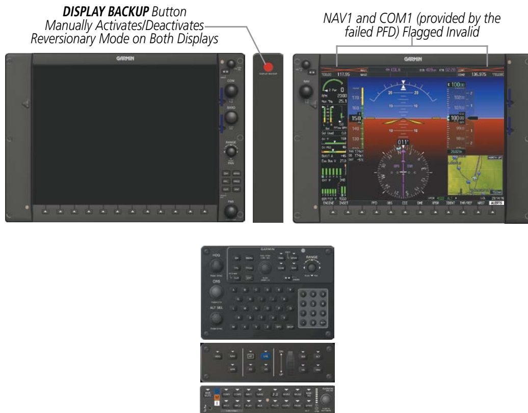
Figure 1-17 Reversionary Mode (Failed PFD)
