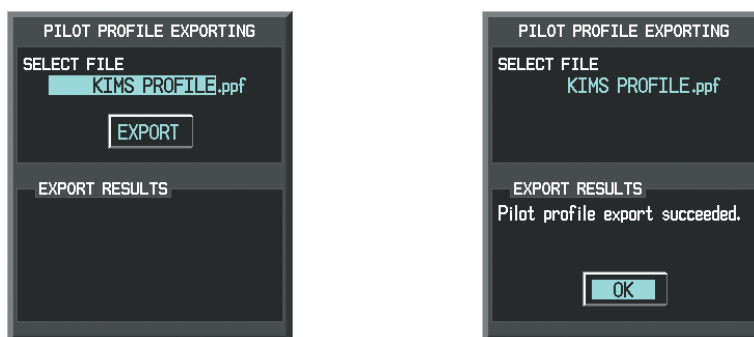
Pilot Profile Exporting Window, Enter a Name to Use for Exported Profile
