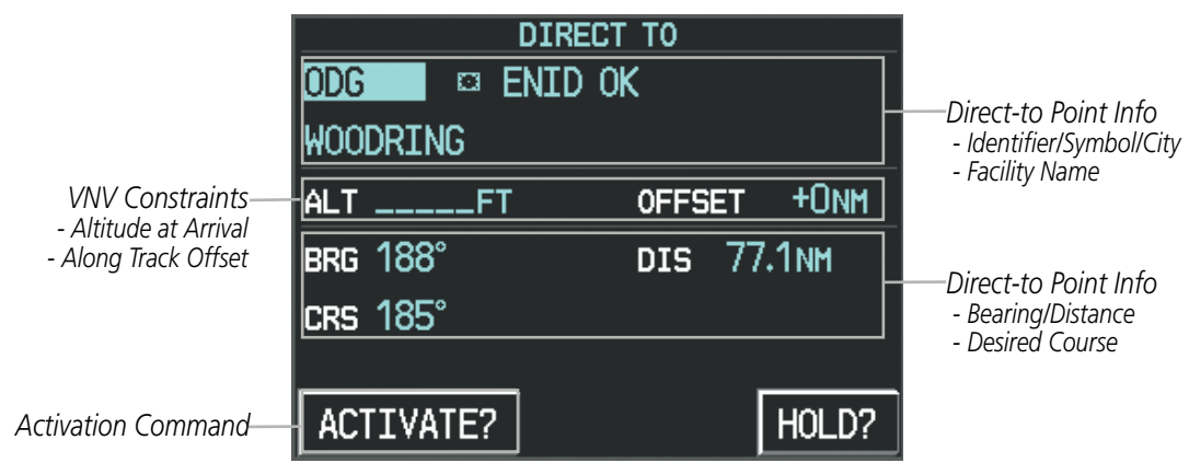
Figure 5-53 Direct-to Window - PFD
