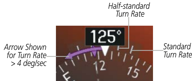
Figure 2-18 Turn Rate Indicator and Trend Vector
